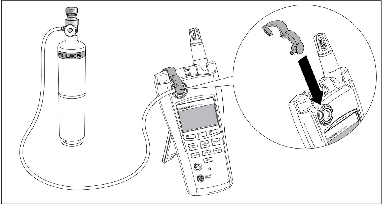
**Figure 4. Calibration Set Up**
