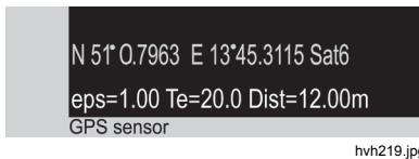
Along with latitude, longitude, and the number of satellites, further GPS information is saved together with the thermal image: height, speed, and bearing.
