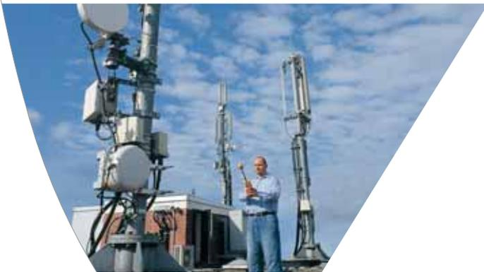
Example: Safety zones around mobile phone antennas. You can easily read off the field strength value, and the device warns you immediately if the limit value is exceeded.
