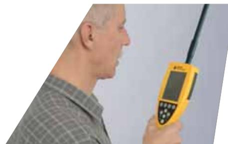
You can record your own voice comments and replay them over the earphone. Each comment is stored with the corresponding measured value. It can be transferred to a PC with the results and played back using the PC's sound card.
