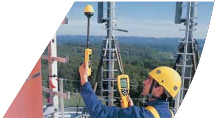
Example: Safety when working on transmitter towers. The field strength can be checked with the probe before you approach the vicinity of the antenna.
