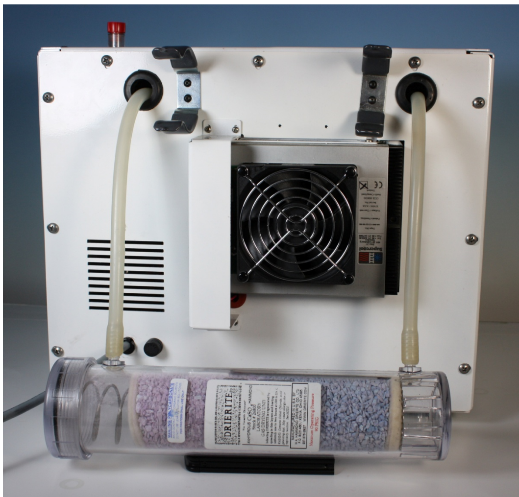
Figure 2: Desiccant Reservoir Pulled From H300
