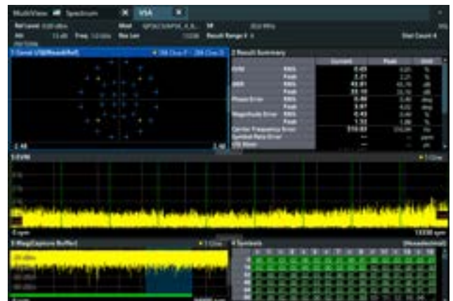
Demodulation of a DVB-SX2 multi-modulation signal with the R&S®FPL1-K70M option (R&S®FPL1-K70 option required)
