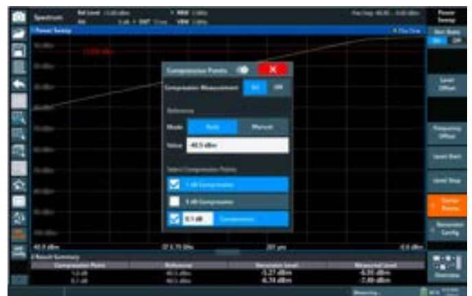
Measurement of 1 dB and 0.1 dB compression points
