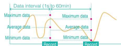
Set the power logger to save all parameters to record the maximum, minimum, and average values during the set recording interval.
