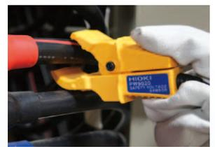
STEP4 Connect the clamp sensors
