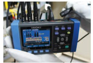
STEP3 Connect the voltage sensor
