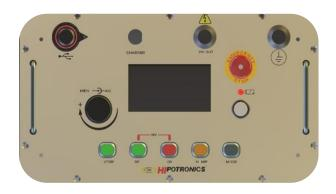
The X-Wave is operated by large, color-coded push buttons and a single rotary knob selector. The MODE button is used to access the main menu.
