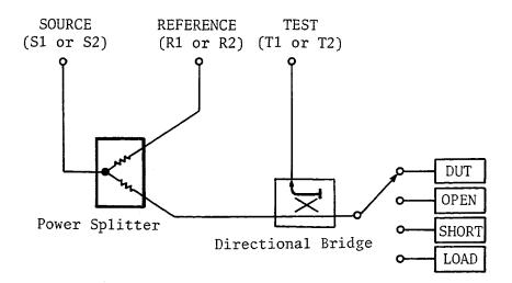
Figure 4-3. Reflection Calibration Diagram
