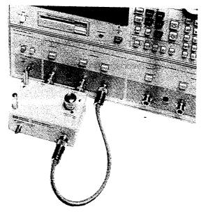
Figure 3-3 shows the impedance test adapter connected to the 4195A.
