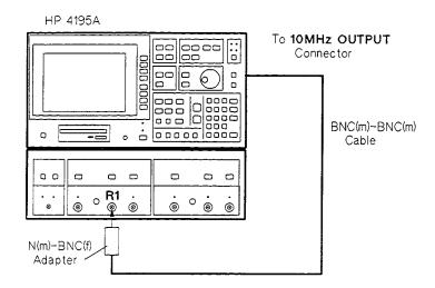
Figure 3-2. Spectrum Measurement Example Setup
