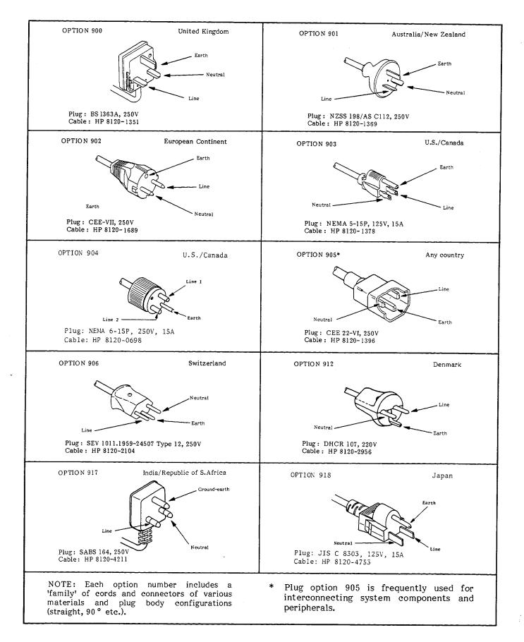
Figure 1-4. Power Cables Supplied
