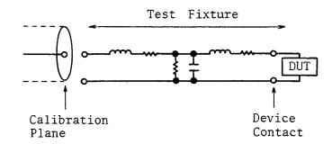
Figure 4-5. 0S/0Ω Offset Compensation
