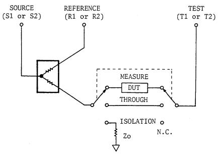
Figure 4-2. Transmission Calibration Diagram
