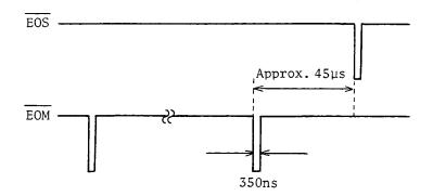
Figure 5-8. EOS and EOM Output Timing (Typical)
