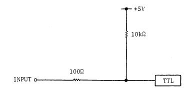
Figure 5-6. 8-bit Input Port Equivalent Circuit
