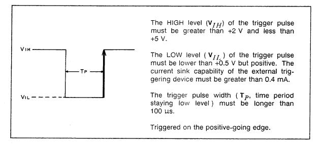
Figure 4-8. External Trigger Pulse
