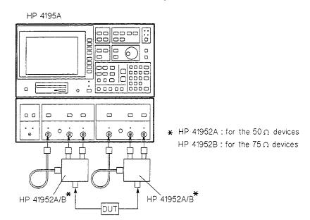
Figure 3-6. S-Parameter Configuration Setup Example
