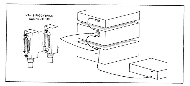
Figure 6-3. Typical HP-IB System Interconnection
