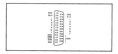
Figure 5-5. 8-bit I/O Connector
