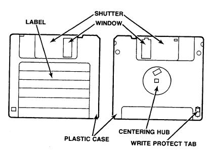
Figure 5-11. Parts of the Flexible Disc
