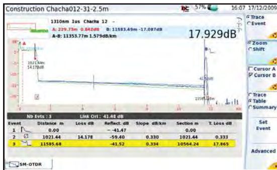
PON system measurement from the customer premises
