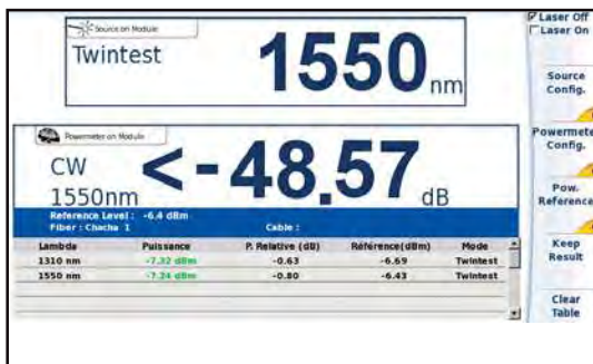
Loss test set feature (light source and power meter)
