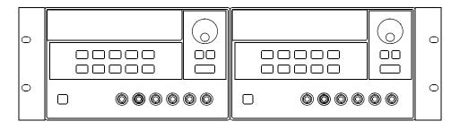
To rack mount two instruments of the same depth side-by-side, order lock-link kit 5061-9694 and flange kit 5063-9214.
