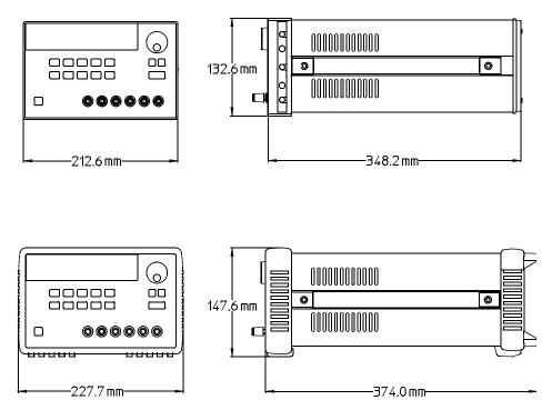
Figure 8-1. Dimensions of Agilent E3631A Power Supply
