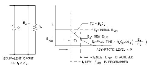
Figure 7-8. Speed of Response -Programming Down
