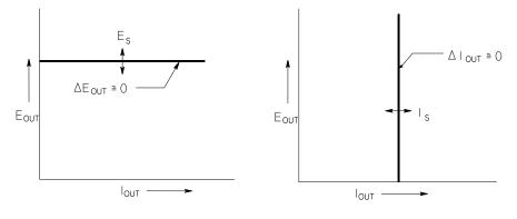
Figure 7-3. Ideal Constant Voltage Figure 7-4. Ideal Constant Current Power Supply Power Supply
