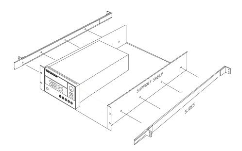
To install two instruments in a sliding support shelf, order support shelf 5063-9256, and slide kit 1494-0015.
