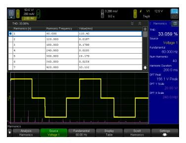
Perform harmonic analysis on voltage or current. Both the time domain waveform (yellow trace) and the harmonic table are simultaneously displayed.
