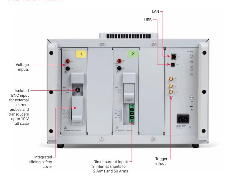
When measuring current with the direct current input, wiring to the DUT is connected on a removable connector, allowing you to quickly remove the wires for fast reconfiguration.
