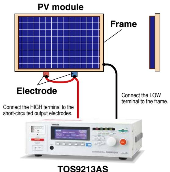
\* The module connection method for PID reproduction is the same as for the insulation tests. By selecting the TOS9213AS insulation resistance test mode (IR), the applied voltage will have negative polarity.
