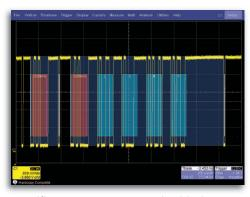
specific events on your embedded controller. Trigger on DATA in specific locations of long I<sup>2</sup>C EEPROM reads, or trigger on sensor values outside of a certain range. Intuitive, color-coded decode overlay helps you understand your serial data signals quickly. Search for data patterns, or view the protocol data in a table. Export table data to Excel. (Capabilities are optional).
