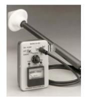
Holaday's HI-1801 provides an easy an inexpensive means for public health agencies and service technicians to check microwave leakage. A durable, compact and portable instrument, the HI-1801 is not susceptible to damage caused by excessive fields.
