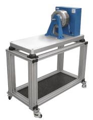
Positioning and alignment have a great influence on the measured parameters (friction torque). MAG-TROL strongly recommends a support specifically dedicated to the products to be tested to ensure the best positioning tolerances in X-Y. and its repeatability.
