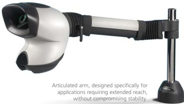
Articulated arm, designed specifically for applications requiring extended reach, without compromising stability.
