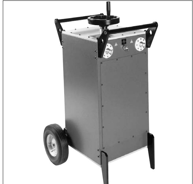
The optional Resonating Inductor expands the capacitance range of the DELTA3000
