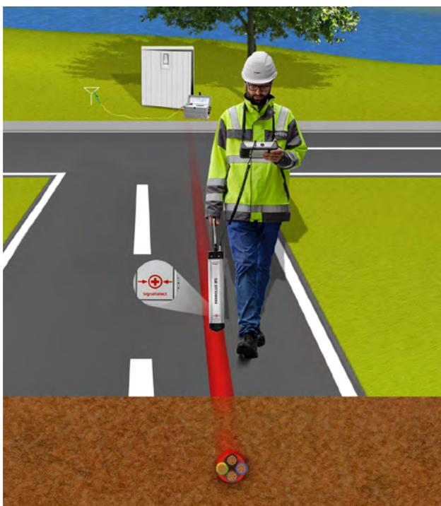
This is all possible thanks to a continuous display of the installation depth and the signal current as well as automatic supporting functions (e.g. minimum turbidity).
