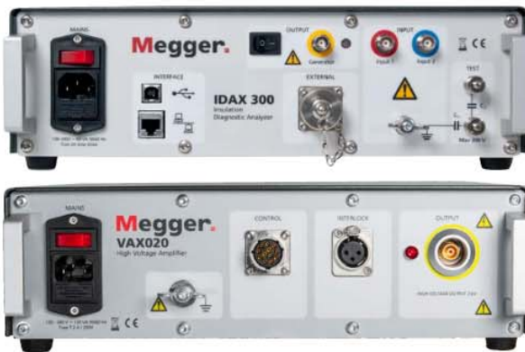
The test system: IDAX-300 and VAX020
