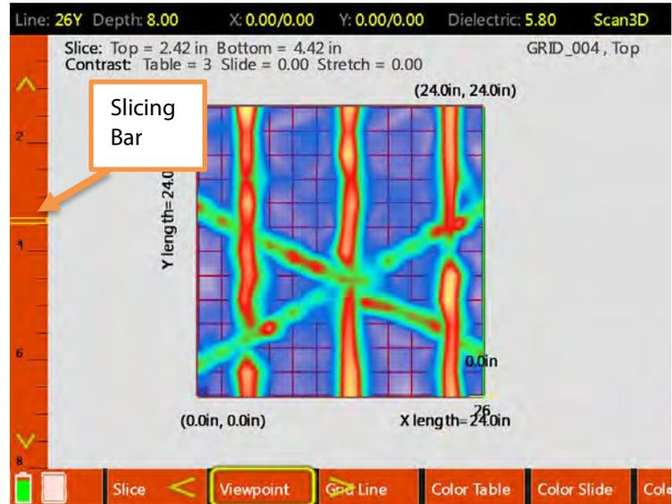
**Drill Hole:** Allows you to position and “drill” a hole into your data set. The hole will display green if considered safe, and red if the system expects the hole to contact a high amplitude signal which could represent a target. This should not be considered as a definitive answer, but rather as an interpretive tool. Do not rely solely on this feature for your interpretations. Please refer to the StructureScan Mini XT manual for details.
