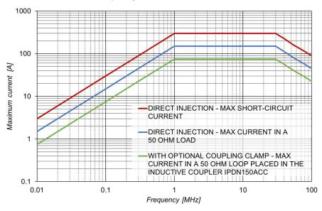
Examples of direct current injections in a 50 ohm load
