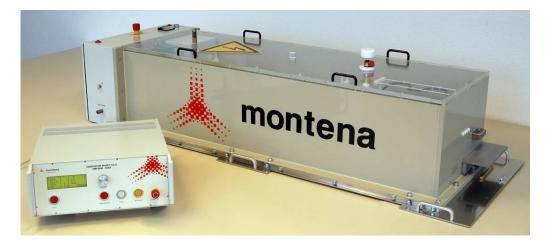
This generator is used to measure the performance of conductive points of entry and of protective devices according to MIL-STD188-125-1/2 (PCI: pulse current injection). It produces double exponential current pulses of short duration up to 5 kA. It can be fully controlled by a computer through a RS232 and USB interface. We provide all the necessary accessories like current probes, coupling and decoupling networks, fibre optic links, etc. The automation software is also proposed as an option.
