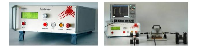
This test generator is designed to comply with the requirements of the MIL-STD-461 CS115. The test method CS115 is used to verify the ability of the EUT to withstand pulse excitation on interconnecting cables. The pulse generator can be ordered with all the accessories in order to build the full test set-up basically consisting of an injection probe, an attenuator and an oscilloscope. The generator can be fully controlled by a computer through a RS232 and USB interface.
