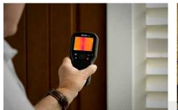
**GET TO THE PROBLEM FASTER** Visually scan and investigate large areas for moisture, air leaks, and other building issues without opening the wall
