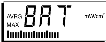
Figure 3-2 Low battery warning: BAT and measurement result displayed alternately
