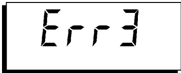
Figure 4-18 An error was detected during the self-test.
