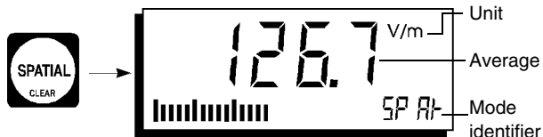
Figure 4-31 “Spatial Averaging” mode for determining the average field strength within a spatially extended area
