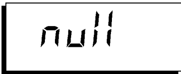
Figure 4-17 Display during automatic zeroing
