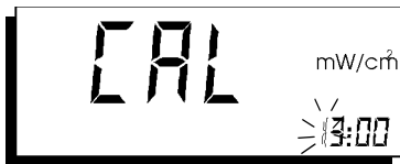
Figure 4-13 CAL display. The calibration factor setting is displayed in the lower right corner. The digit which can be altered flashes in the display.
