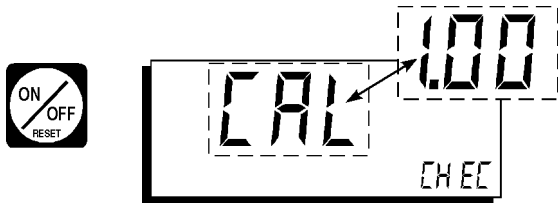
Figure 4-4 The self-test runs immediately after switch-on
