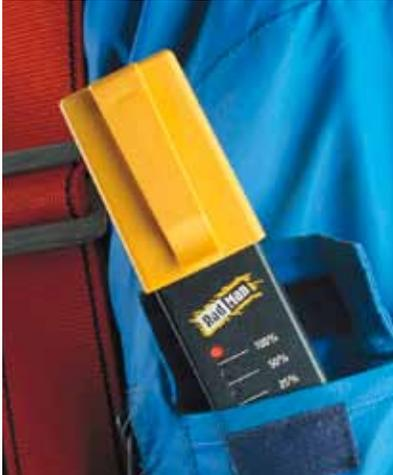
Personal monitors are best worn on the outside of clothing or in your outside breast pocket (though not in the outside pocket of very heavy clothing) and lying flat against your body. Absorbers minimize the influence of the body. The absorber for the RadMan / RadMan XT is located in the yellow protective cap. The absorber for the Nardalert S3 is an integral part of the housing.
