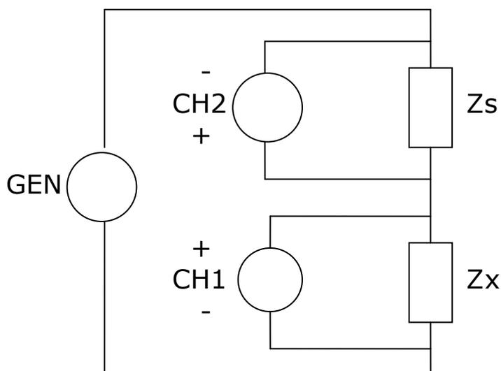
For “shunt” connection, shown above, the current is measured directly across the shunt using CH2 while the voltage across the  $Z_x$  is measured by CH1. Notice that the positive inputs to both CH1 and CH2 are connected to the midpoint to minimise common mode loading effects.
