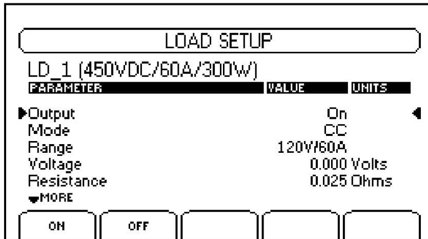
**1. OUTPUT** - allows you to toggle the module's ON/OFF state as well as the state of its isolation relay if installed.
