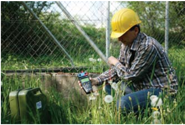
Touch Voltage Measurement Using the CP AL1, CPC 100 and CP CU1
