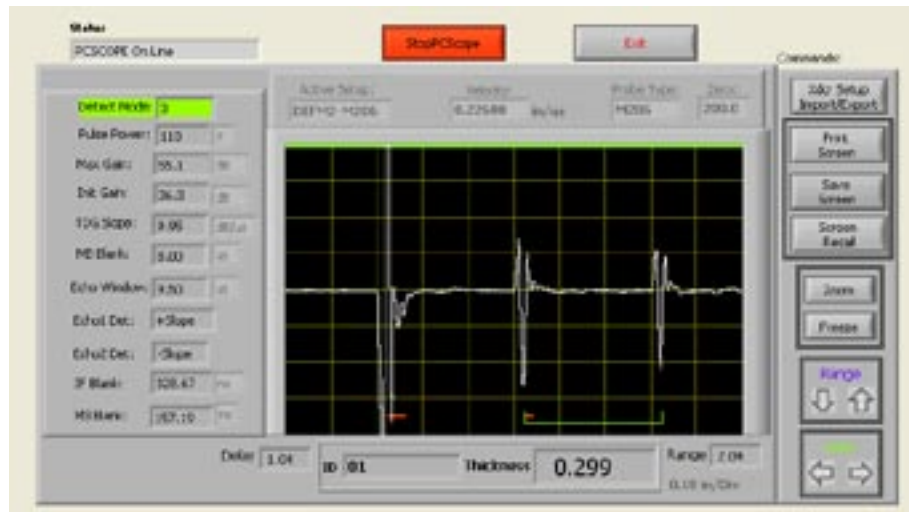
Thickness and waveform of a very thin (0.004 inch or 0.10 mm) sheet of steel.
