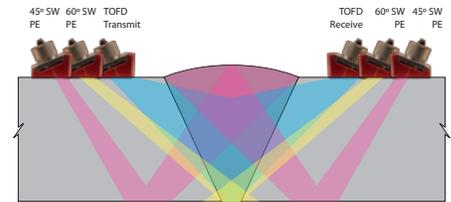
Weld inspection using combined TOFD and pulse echo (PV-100).
