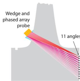
Multiple-angle inspection with one multielement probe.
