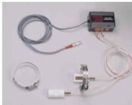
Dual RTD transmitter and RTDs.
