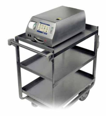
The MET ONE 3411 is designed to meet the rigorous requirements of ISO-21501-4 to provide the users with unparalleled accuracy. This ensures the repeatability of particle measurements between multiple instruments; critical for process benchmarking and troubleshooting activities.
