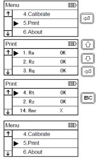
Here you can select, which parameters shall be printed out. To do so, select the particular parameters by using the arrow buttons and and press the "Enter/menu" button afterwards. "OK" means that the selected parameter appears on the printout. "X" means that the parameter does not appear on the printout.
