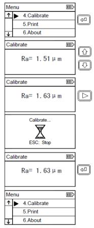
Use the arrow buttons and to adjust the Ra value on the screen to the properties of the calibration standard. Once you are done, press the "Enter/menu" button to confirm.
