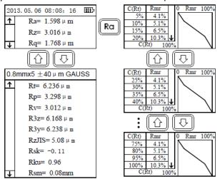
If a printer is connected to the device, you can print out the selected record by pressing the "Save/print" button .
