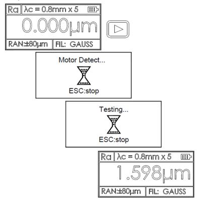
The stylus moves along the measuring distance and back to its starting position. After that, the readings are shown on the display. Use the "Parameter selection" button to view further measuring parameters.
