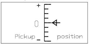
The stylus position is ideal when the arrow indicates "0". Use the adjustable support to adjust the stylus position.
