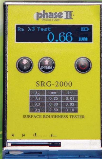
The SRG-2000 determines surface roughness parameters Ra, Rz, Rms(Rq) and Rt within a wide measuring range. The piezo-electric pick-up stylus with diamond tip assures a very reliable measurement within tolerances that conform to ASME B46.1. Surface Roughness parameter Ra is computed to conform to ISO and Rz is computed to conform to DIN.
