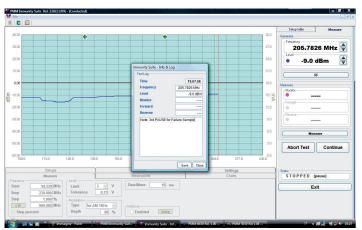
Pause during the frequency scan at EUT failures and Manual Adjustament of both Frequency and Level to identify hreshold of sesceptibility
