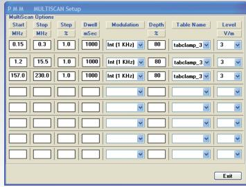
Multi-Scan Table to perform test only on most critical frequency's segments and save time during debugging phase
