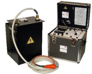
Shielded output cables have their limits and grow too large and inflexible at higher voltages and can consume too much of the limited output power (in the case of ac hipots).
