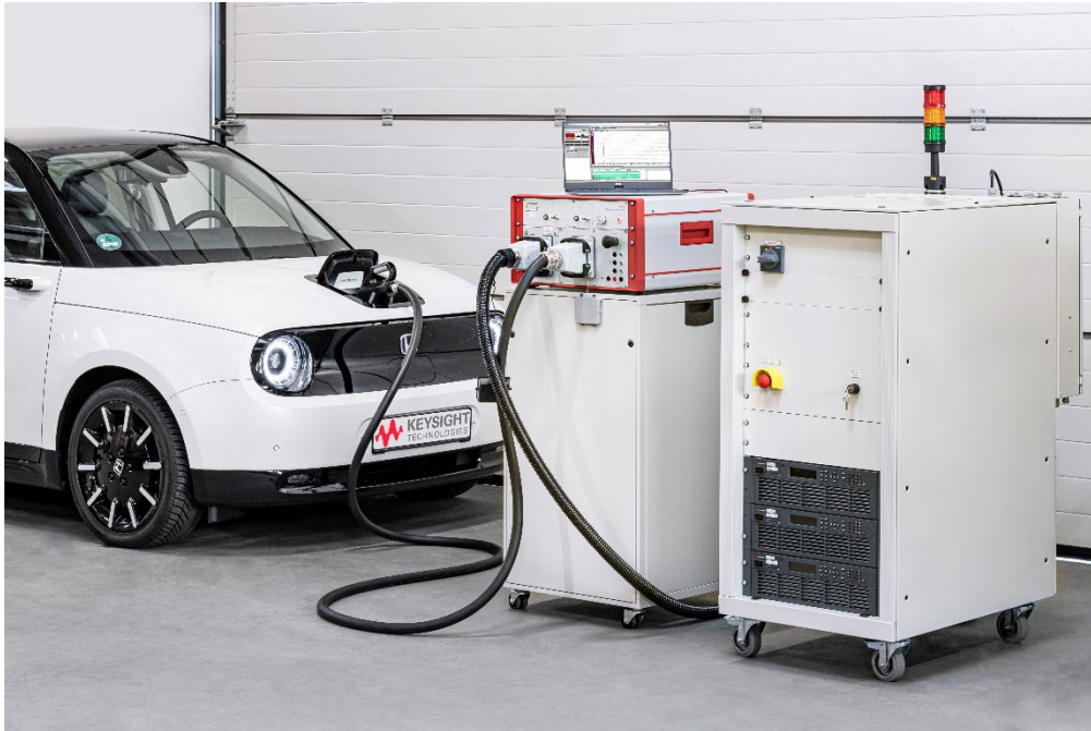
Figure 10. AC charging test with SL1214A Dual-Range AC Emulator and SL1040A Charging Discovery System test.
