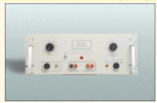
For those who have graduated from the 50 volt and 100 volt spike susceptibility category, we offer this high-power 600 volt transient generator. The **Model 7054-1** delivers over 300 kw into low resistance loads. It has the flexibility and capability of the previous models, including the ability to shift the transient in phase to any position on the sine wave of the a.c. line feeding the test sample. The amplitude and the repetition rate are adjustable.
