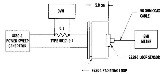
FIG. 4b TEST SETUP FOR CURRENTS GREATER THAN 25 mA
