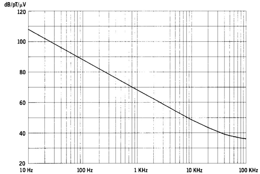
FIG. 2 CORRECTION FACTOR, TYPE 9229-1 LOOP SENSOR
