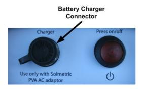
Charging the battery can take up to 6 hours. Once the battery has been charged, the PVA-600 will operate for approximately 2 days of normal use. During heavy use, nightly charging is suggested.
