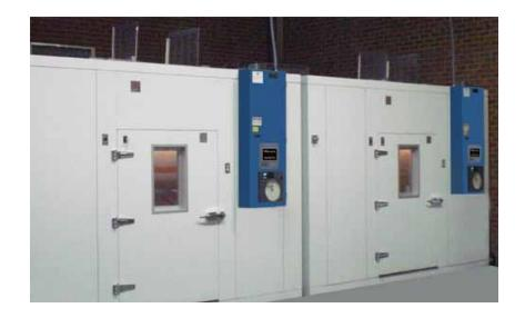
This room is designed to store bottles of pharmaceutical product at -70°C. With over 4800 cu.ft. of conditioned interior space, the chamber is divided into four zones that can each hold up to 288 bottles.
