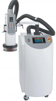
The DC controlled ThermalAir TA-5000 System power adjust almost instantaneously to your temperature settings and test conditions real time. Providing percise temperature control when you need it while saving energy.
