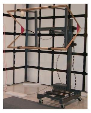
The TDK EFG-03 E-Field Generator generates controlled, high intensity fields over the operating range of 10 kHz to 100 MHz.
