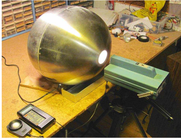
Figure 3: Light Integrating Sphere
