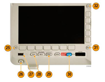
**29. Default Setup**. Push to perform an immediate restore of the oscilloscope to the default settings.
