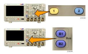
2. Push a lower-bezel button to create a label, such as for channel 1 or B1.
