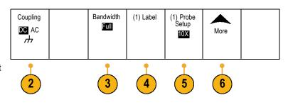
3. Push **Bandwidth**, and select the desired bandwidth from the resulting side-bezel menu.
