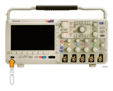
**4.** Power on the oscilloscope. The oscilloscope automatically recognizes and installs the replacement firmware.
