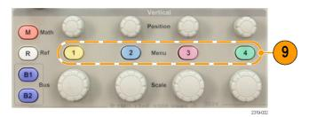
10. B1 or B2. Push to define and display a serial bus if you have the appropriate module application keys. The DPO2AUTO module supports CAN and LIN buses. The DPO2EMBD module supports I<sup>2</sup>C and SPI. The DPO2COMP module supports RS-232, RS-422, RS-485, and UART buses.
