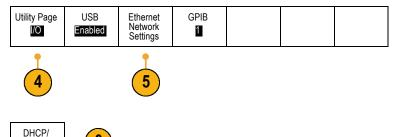
Push Change Instrument Settings. If you are using DHCP, note the Ethernet address and instrument name. If you are using Static addressing, enter the Ethernet address you will be using.
