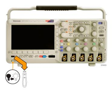
6. Power on the oscilloscope.
