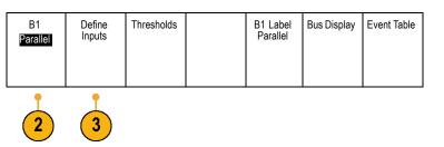
Use the side-bezel buttons to define parameters for the inputs, such as specific signals to an analog or digital channel.
