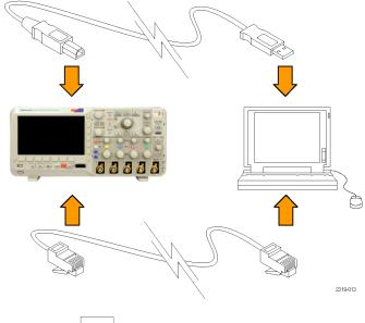
To communicate between the oscilloscope and a GPIB system, connect the oscilloscope to the TEK-USB-488 GPIB-to-USB Adapter with a USB cable. Then connect the adapter to your GPIB system with a GPIB cable. Cycle the power on the oscilloscope.
