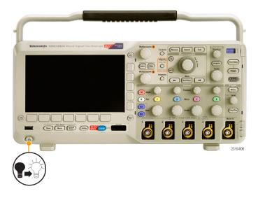
3. Connect the P2221 probe tip and reference lead to the **PROBE COMP** connectors on the oscilloscope.
