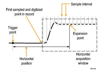
■ Trigger point: The zero time reference in a waveform record. It is shown on the screen by an orange T.
