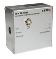
Impedance stabilization networks (ISN) are coupling/decoupling networks according to CISPR 22 (EN 55022) for measurement of conducted common mode disturbances of information technology equipment (ITE). The ISN is placed between the equipment under test (EUT) and the auxiliary equipment (AE) or load which is necessary for the operation of the EUT. The ISN establishes the common mode termination impedance seen by the telecommunication port during measurement.
