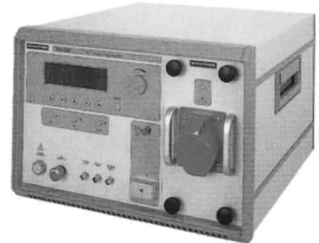
Any of the saved, pre-programmed or custom tests can easily be combined into a sequence for automatic execution. When the sequence is run, WIN 2025 executes each of the tests in turn, without any need for further operator intervention. This allows engineers to optimise test procedures and to manage laboratory test time efficiently for maximum throughput.
