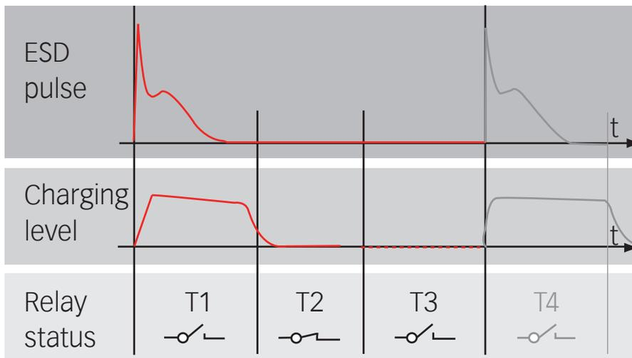
All times are individually and freely adjustable from 0.1 to 99 s in step sizes of 0.1 s. The sum of the three time segments gives the pulse repetition rate.
