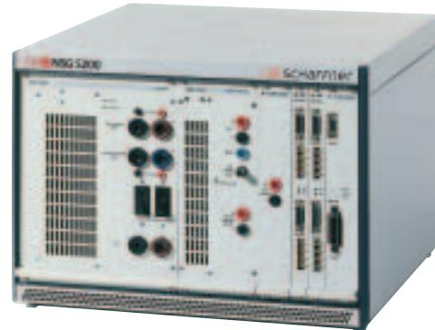
**Basic Chassis NSG 5201 and NSG 5202.** The 19" basic chassis contains all the power supply components and, if required, the burst-transformer, the rear-facing fans, the control and signal bus boards as well as the common inputs and outputs for the safety circuits and signals for the expanded control and monitoring of the test procedures.
