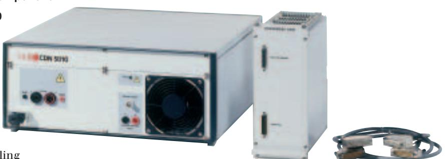
The high current coupler type CDN 5010A, equipped with both a switch and decoupling filter rated at 60V and 60A, is controlled by the system controller. The pulses are fed to the CDN 5010A via a cable from the output on the generator module in the System NSG 5000 and are superimposed on the battery voltage. All the functions, such as battery
